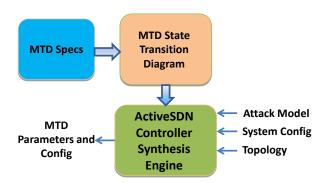
**Figure 4: MTD Controller Synthesis**
